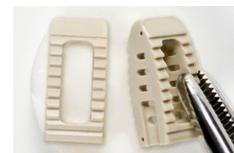
VESTAKEEP® iC4620 3DF is an opaque, medium viscosity polyether ether ketone (PEEK) filament. It contains 20% carbon fiber to enhance stiffness.
